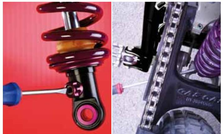
We adjust extension or rebump with this setting. There are 50 clicks available. The starting position by default is centered at 25. By screwing the golden vise clockwise we will slow the extension, and the bike will be slower, if we unscrew it (opposite to clockwise), we will unleash the extension, and the bike will be faster. In order to be able to perceive the change in the setting, it is recommended to change 3 clicks every time. Fine tuning must be done from 1 click to the next one.
